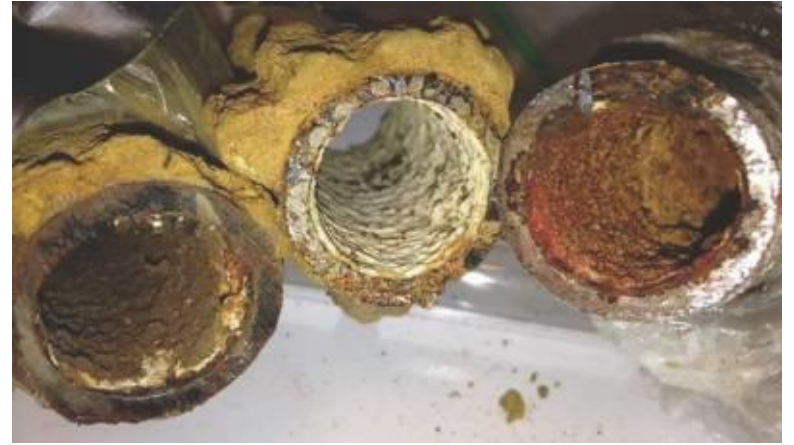
Pipes from the Flint water distribution after the city switched the water source to Flint River
